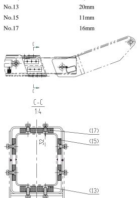
3. If the thickness smaller than the illustrate size, please change the slide block. In the whole movement range, checking the telescopic boom may be cause the main part
